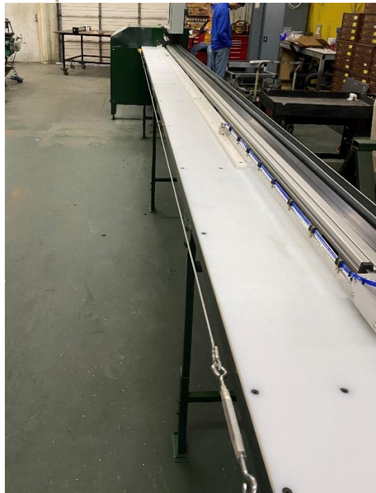
Figure 1: Current Infeed Table and Pusher
