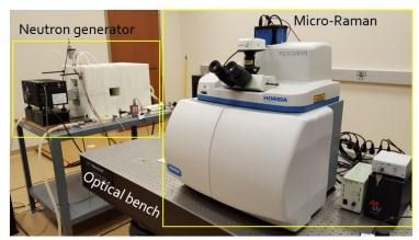
Figure 1: Photograph of the neutron source and micro-Raman instruments
