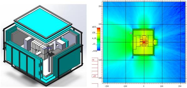
Figure 2: Shielding of neutron source for user operation; exploded view of solid model of shielding design (left) with high density polyethylene HDPE (white), boronated polyethylene BPE (blue), and steel (black), Monte Carlo simulation of radiation outside of the shielded enclosure (right). The green region indicates doses of less than  $2 \mu$ Sv/hr at a distance of 30 cm form the enclosure.
