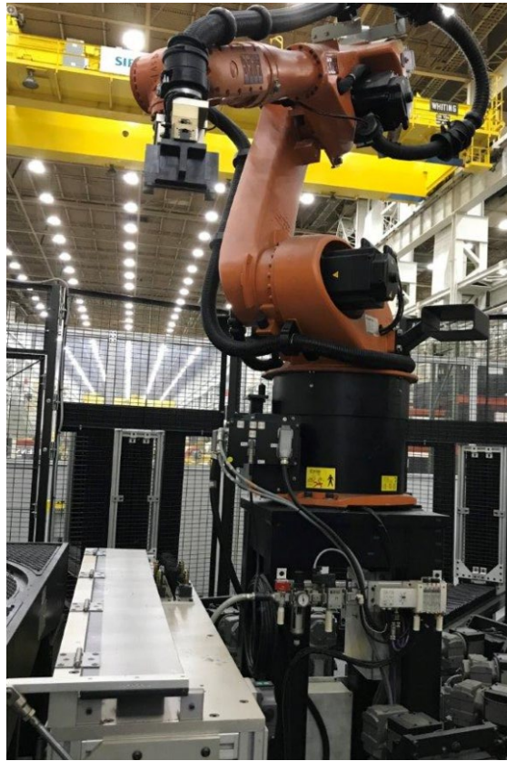
Figure 1: Kuka Robot with fixturing and clamping example shown.
