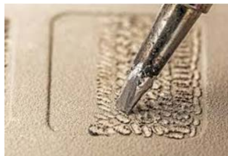
Figure 2: Hand Stippling a polymer surface.
