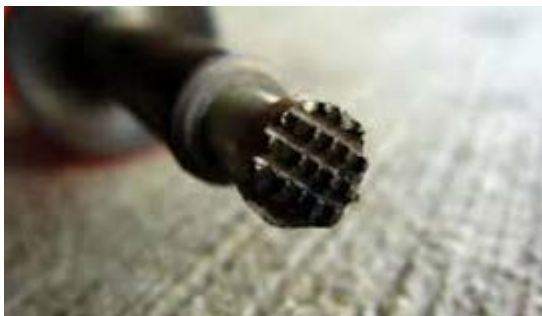
Figure 1: Stippling Head on Solder Iron
