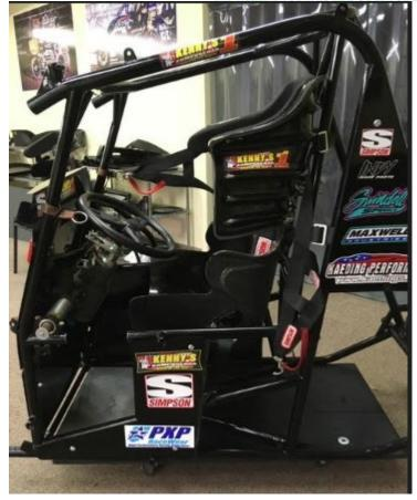
In designing this project safety, weight and space must all be factored in. The cockpits of these cars are extremely confined so the design must take that into consideration. Race cars are designed to be as light as possible so any design needs to be lightweight but strong. The primary focus with this is safety. Drivers who sit at 90° are at more risk of suffering severe back trauma. The objective of this project is to lower that risk with the design of a safer mounting system.
