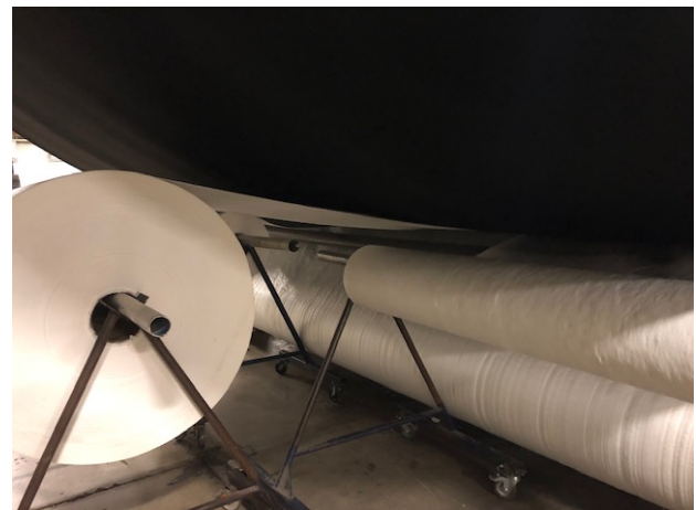
Material Set Up in Machine: Rolls are close together causing issues when changes occur and when replenishing material.
