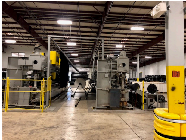
Side view of entire machine 1: Material sits in-between two needle punching lines. Shown is three different material layered together
