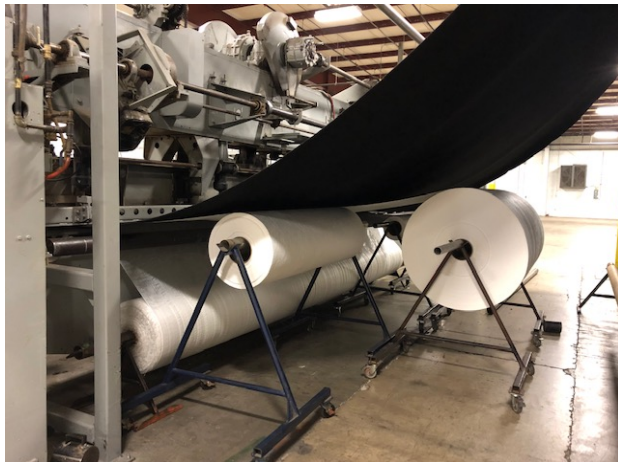
Material Feeding into Machine: Different materials, lengths and sizes of rolls. All being pulled through the machine
