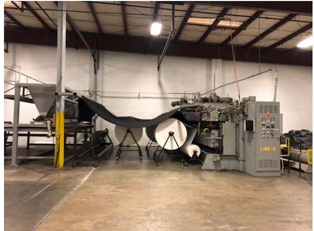
Side view of entire machine 2: Material sits in-between needling line and material hopper. Multiple rolls side by side to get desired width.
