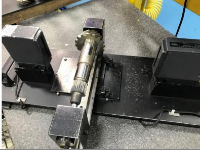
In a typical day, approximately 7000 gear sets (ring and pinion gears make up a gear set) are inspected. A variety of inspection methods are used (go/no go gages, laser measurement, etc.)
