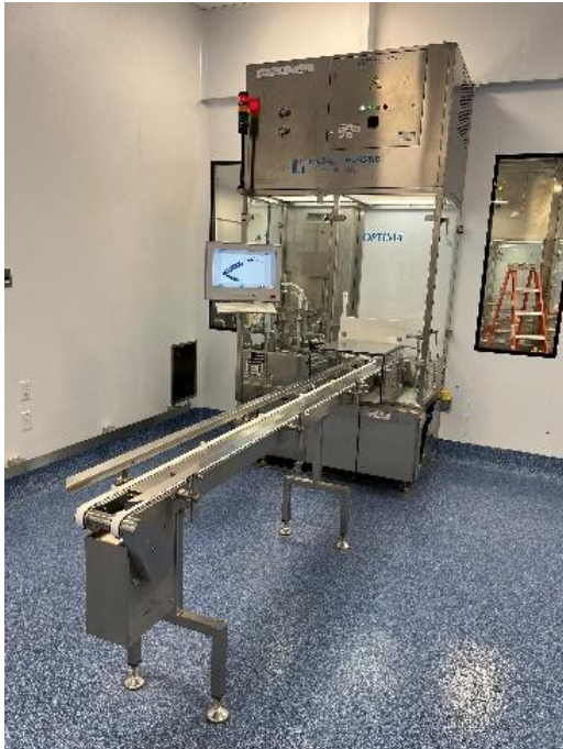
Example 3: Loading Conveyor and DBA-S system
