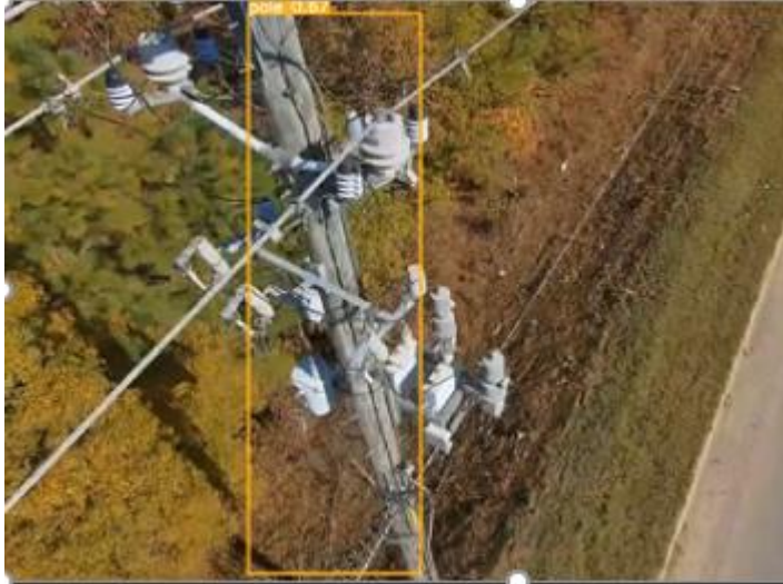
Figure 2 Yolov5 Pole class, object detection
