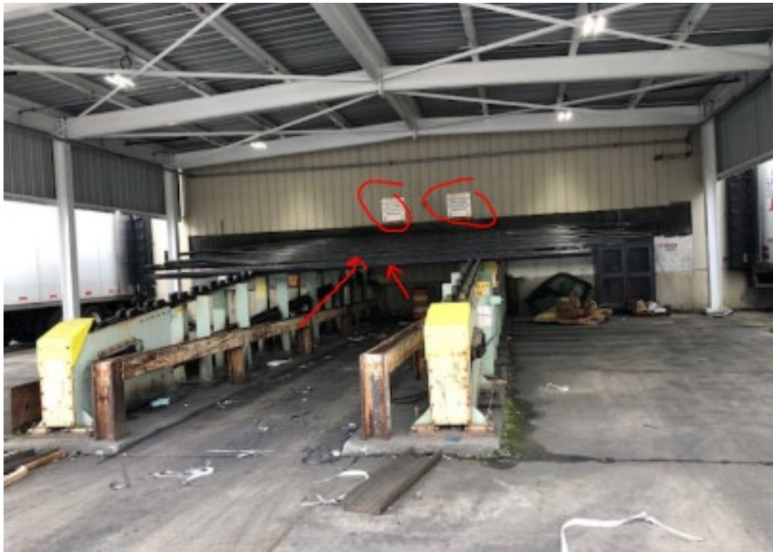
Figure 2 – Conveyor that transports frame rails into building to the “Denester” station
