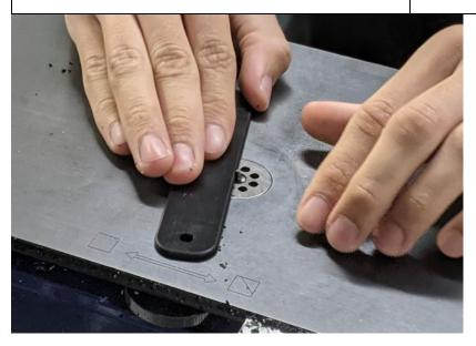
This operation is very repetitive and lends itself well to being automated. The objective of the project is to design a way to have the beveling operation done by a machine. Team will survey the products that need this treatment and design a prototype automated machine that can accommodate different shape parts that are the same thickness. Parts accommodated will be based on what can be done within the team's budget and schedule.
