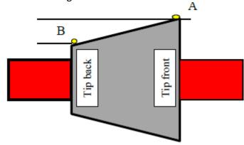
If the angle is not ground correctly, it will lead to quality of cut issues. The distance between
