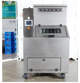
We hope to continue improving our system in ways that make it more feasible to implement world-wide. The current system utilizes a single passive manifold for dispensing water into the bottles. Filling volume is controlled by regulating the system pressure and the filling time. We hope to be able to modify the system so that each bottle can be filled independently and that flavor concentrates or other additives could be added to the bottles in a controlled manner.
