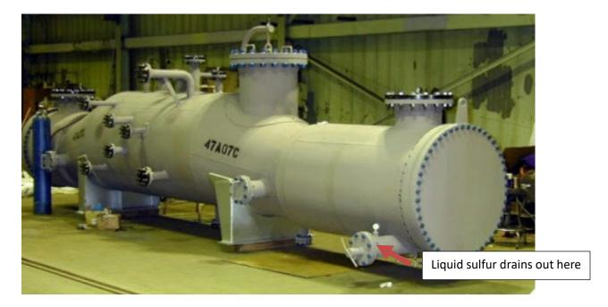
From the condenser, the sulfur is piped through a transition device that separates the high pressure section of the condenser from the atmospheric sulfur storage container which can be an in-ground pit or a tank. This transition device is called a "seal".
