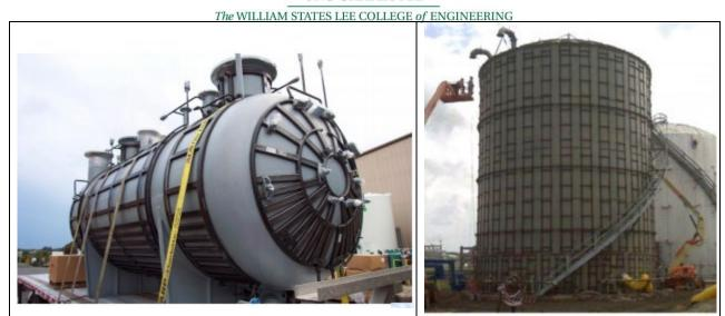
In oil and gas refining, it is necessary to remove sulfur from the refining stream to comply with environmental regulations that help to prevent "acid rain". The oil stream is processed in a refining process to strip out sulfur in the form of Hydrogen Sulfide. Hydrogen Sulfide is sent to a unit called the Sulfur Recover Unit or SRU. The H<sub>2</sub>S is deconstructed into Sulfur in a liquid form that drains out of a Condenser – see process diagram below:
