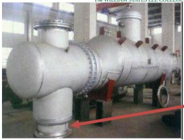
Liquid sulfur drains out here
