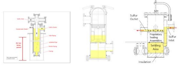
The piping between the condenser and the sealing device is called a run-down line. In most applications, there is not much vertical drop between the condenser outlet and the sealing device. When CSI designs a system, they need to ensure the geometry of the piping system is adequate to accommodate the sulfur flow and process equipment requirements. This project will help improve this design process.
