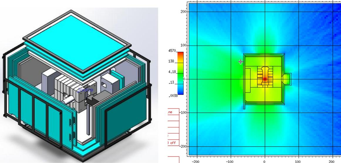
Figure 2: Shielding of neutron source for user operation; exploded view of solid model of shielding design (left) with high density polyethylene HDPE (white), boronated polyethylene BPE (blue), and steel (black), Monte Carlo simulation of radiation outside of the shielded enclosure (right). The green region indicates doses of less than 2  $\mu\text{Sv/hr}$  at a distance of 30 cm from the enclosure.
