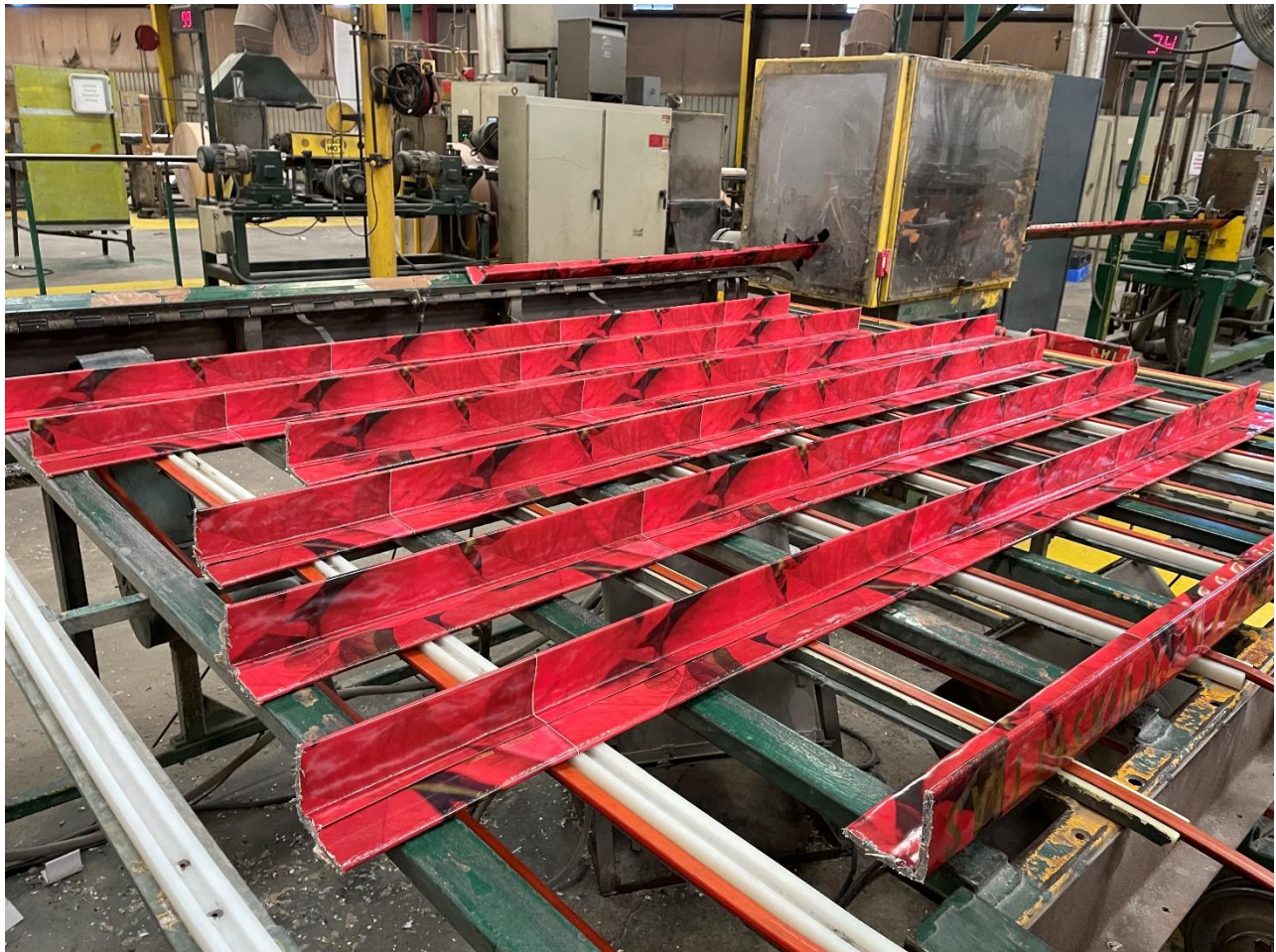
Figure 3: Cutting device (inside yellow box) and downstream cooling table for freshly cut corner boards.
