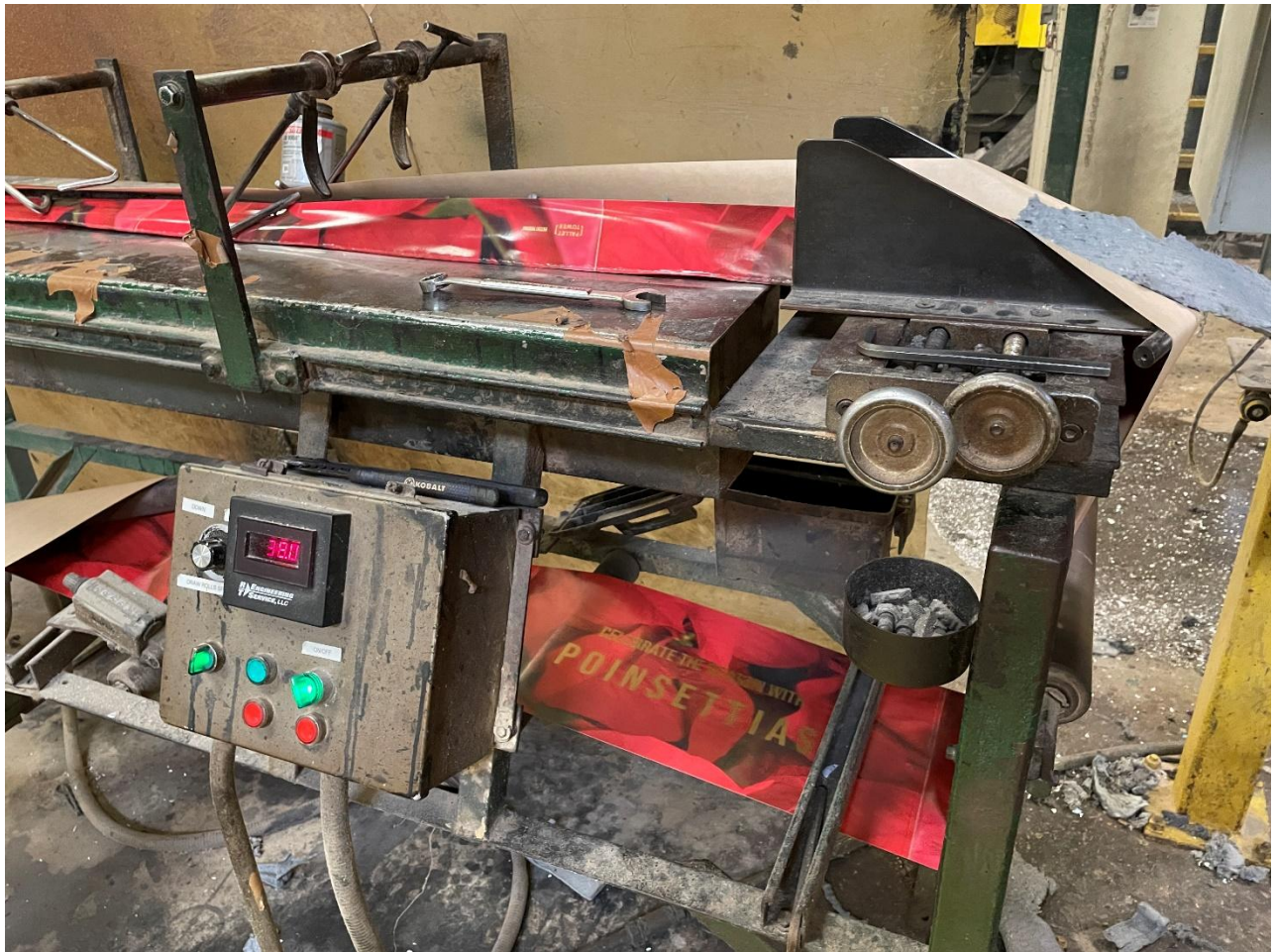
Figure 2: Layering the molten paper/plastic composite into the kraft paper facing.
