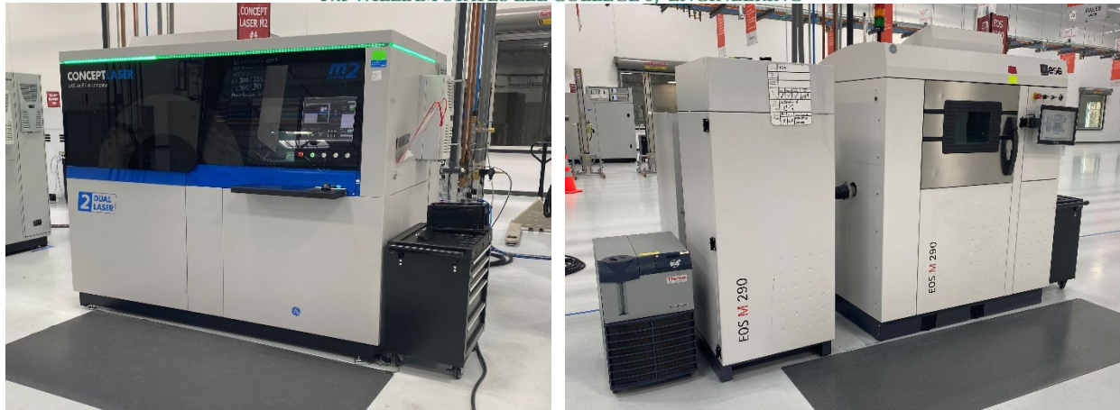
Photographs of a Concept Laser M2 (left) and EOS M290 (right) PBF-LB machines
