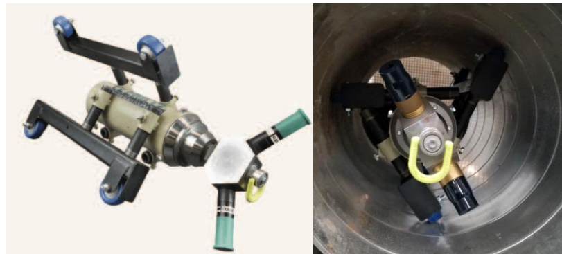
Figure 2: Abrasive Blasting Skid – Pipe Cleaning
