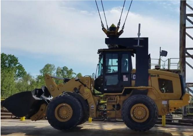
These photos show a lifting frame that Caterpillar developed to allow the crane to pick-up the loader and place it in and out of a barge. The crane lowers the collar device onto the vertical guide pole. When lowered sufficiently, the crane operator remotely actuates pins (see arrow below) that project outward from the pole and retain the lifting collar during the lifting operation. This actuation is done by an air compressor driven actuator.
