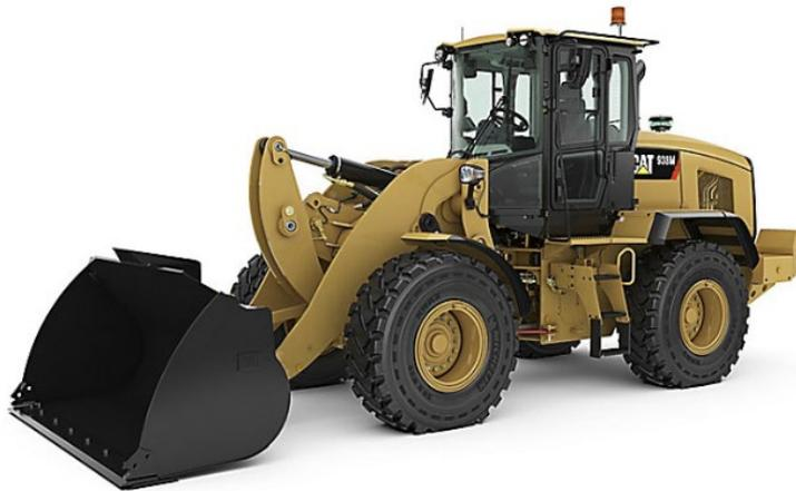
This loader is extremely versatile and is used in many applications. One application is to unload granular material from river barges.
