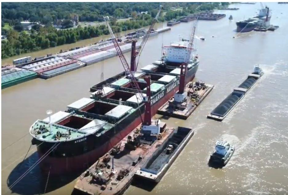
In the picture above, a river barge is being unloaded and the load transferred into a larger ocean going vessel using an overhead crane with a large scoop mechanism. After a certain amount of material is removed from the barge, a Caterpillar front end loader is actually placed inside the barge. The loader moves remaining material into piles that the crane scoop can pick-up. This is repeated until the barge is emptied.
